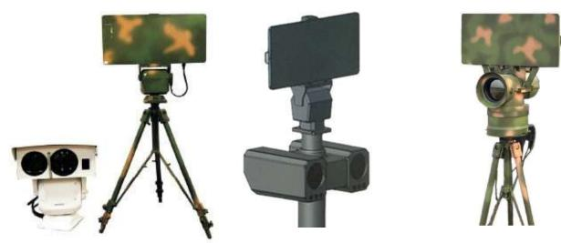
BCS03 consists of the front-end sensor (RF, EO/IR camera) and the back-end control system. The front-end sensor is mainly composed of radar, EO/IR system, controller etc. The back-end system consists of computer and monitoring/processing software. The radar detects targets in the specific range, transmits the detected target information to the monitoring terminal, and display on GIS system.
