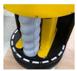
The internal surface is checked by the optical triangulation gauge. The gauge scans needed cross-sections according to a chosen scenario.
