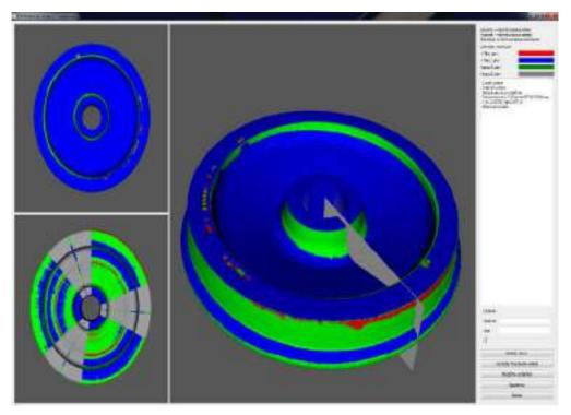
image. The selected cross-section is drawn in the measurement window (on the right monitor). It is possible to load the previously measured wheel offline from the archive.
